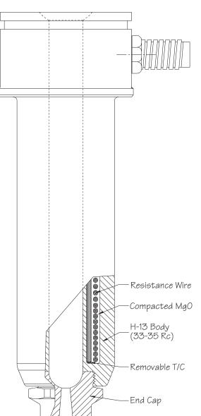
Constructed out of H-13 tool steel.
